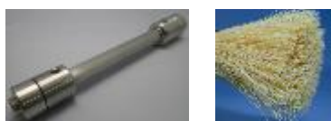
Figure 1 UBE CO-0302SES membrane module for CO 2 separation.
